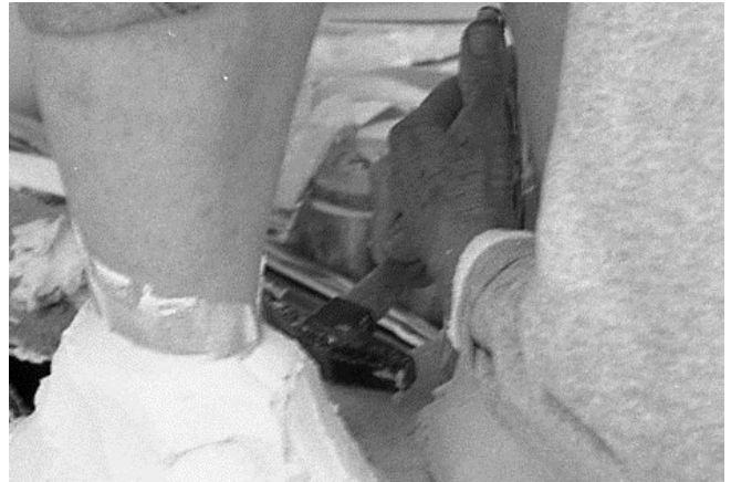
59 The "blunt" butter knife is inserted into the back separation between the two upper plaster halves. A mallet is tapped lightly against the "blunt" butter knife until the two plaster halves come apart.
