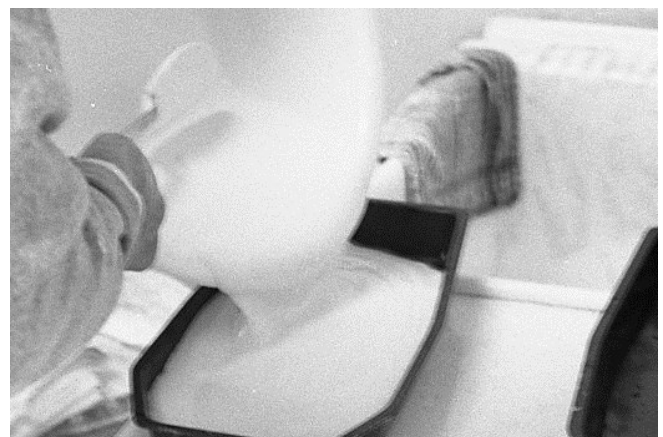
39 After stirring to a uniform consistency, the plaster is placed into a clean pan.
