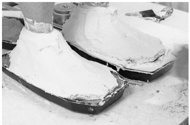
45 The excess plaster which squished out from under the top plaster, has been removed and cleaned away.
