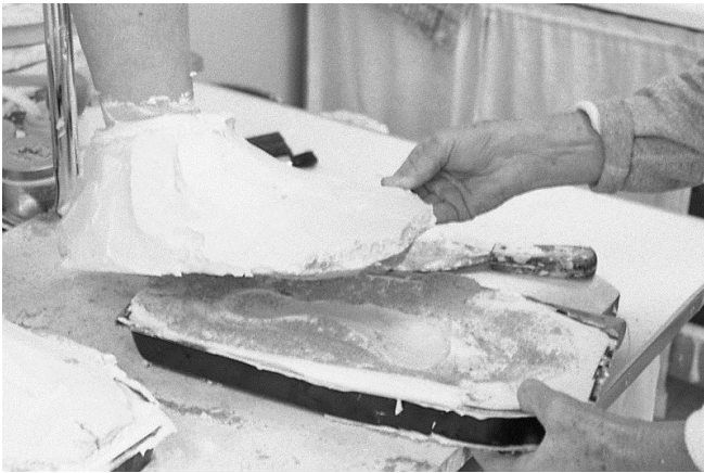
58 The lower pan of plaster is removed.
