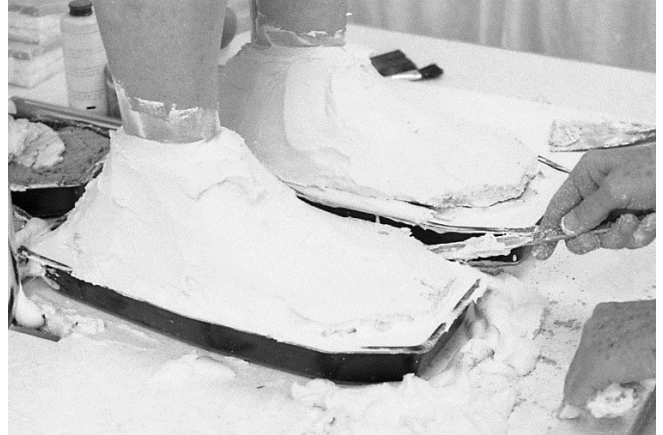
53 The ditches are being made in the bottom plaster.
