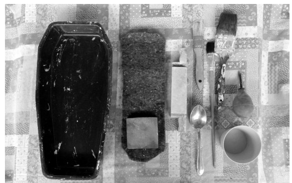
10 The tools and parts of the casting platform on which the foot rests in the plaster casting method. The 1/4" felt is placed in bottom of pan. The 3"X3"X5/8" heel block is placed on top of the felt so as to be under the heel bone. Moist sand, which is not shown, is shaped with the wooden sand shaping tool. See page 5 to view the completed pans of sand.
