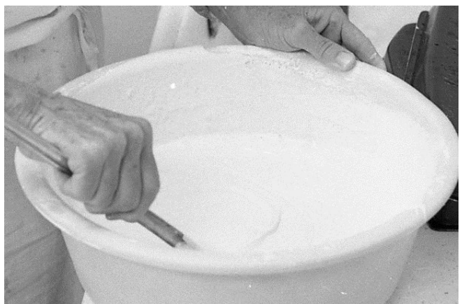
15 After about 5 minutes when the plaster has stopped bubbling, 1 table spoon of salt is added and everything is stirred together until a nice creamy consistency is achieved.
