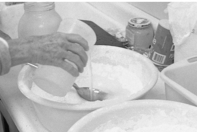
14 Approximately 7 cups of loose and dry plaster is fluffed and placed into a pan. Then 1 1/2 quarts of COLD WATER is added. The COLD WATER helps to moderate the rise in temperature as the plaster hardens. PLASTER GETS HOT.
