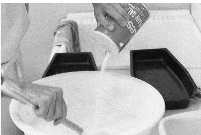
38 After about 5 minutes when the plaster has stopped bubbling, about 3/4 of a tablespoon of salt is added just before the stirring begins.
