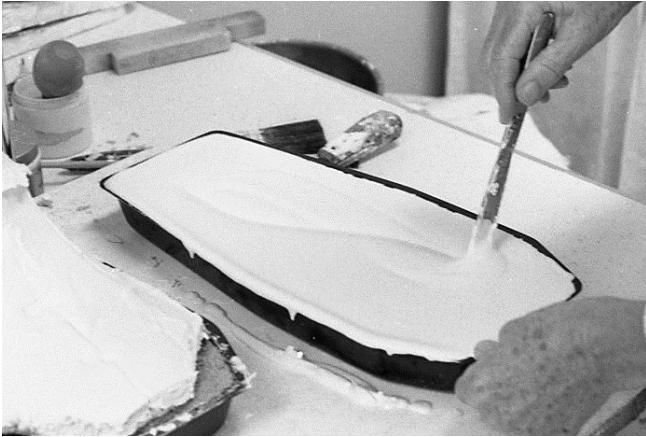
40 The bottom pan of plaster is stirred with the butter knife until it is just about ready to start firming. As shown in the picture, the plaster maintains a slight slump as the butter knife is pulled through the plaster.
