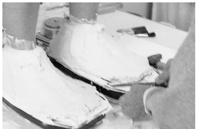
57 After the plaster has firmed enough to become solid, a long screwdriver is inserted into the tunnel and ditch holes. The caster carefully pries the bottom and top plaster shells apart.
