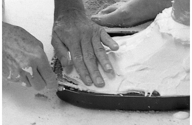
25 The "blunt" butter knife is slid on its side just under the still soft but firming plaster and pushed upwards to make a tunnel for later separation of plaster pieces.
