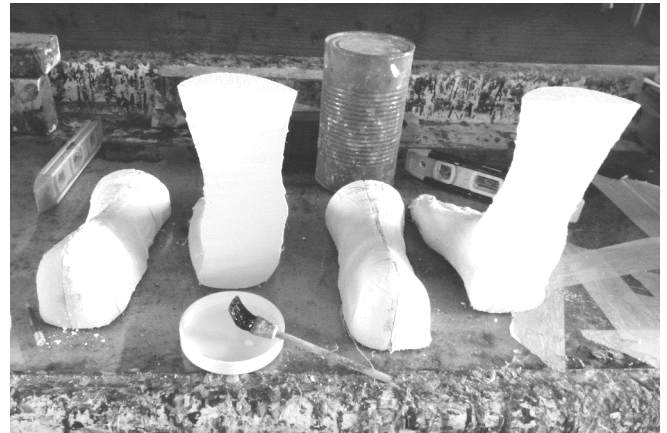
20 Glue is applied to the parts. The backs are glued together using the glass surface for one plane of alignment. After the backs dry, they are glued to the fronts.
