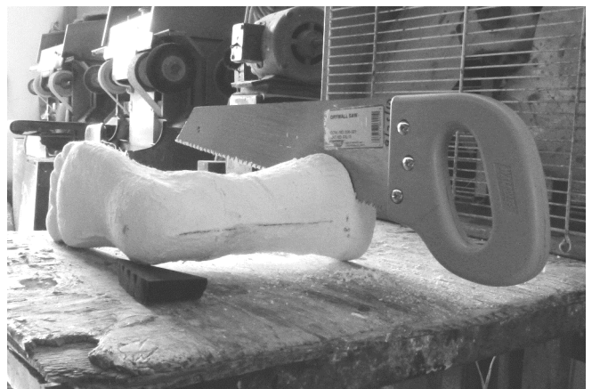
4 Cut the top off above the expected finished height of the boot.
