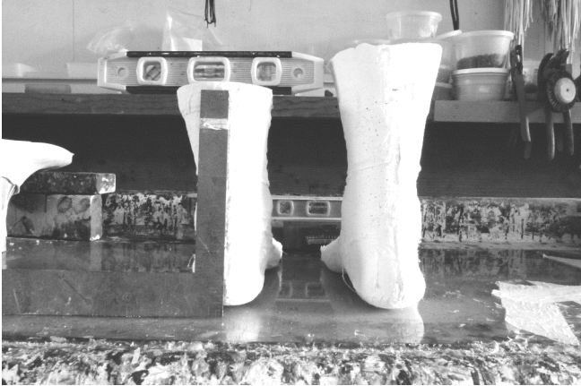
5 Get the alignment with the glass surface correct! Then sand the top of the cast to match the levelness of the glass surface.
