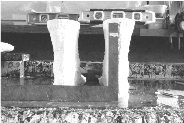
7 Get the alignment with the glass surface correct! Then sand the top of the cast to match the levelness of the glass surface.
