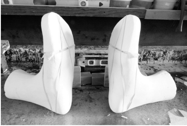
47 I put the new splints in place and control the alignment of the toe to ball and ball to heel angles better.
