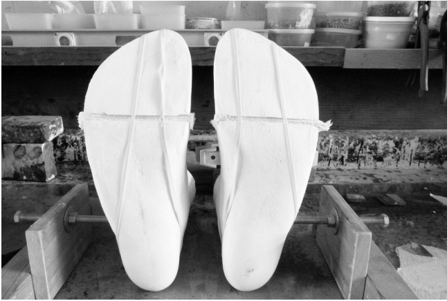
41 Depending on the individual person, 10 or 15 or 20 plaster splints have been added to the length of the ball area plus 3 for the width of the hack saw blade.
