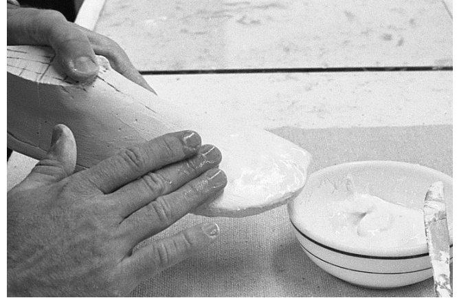
92 Wet fingers are the best smoothers of wet plaster. You control the final shaping with your fingers.
