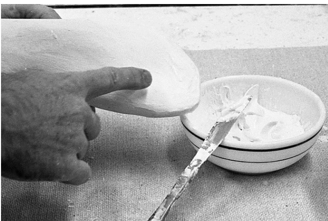
95 This is the area called the "pyramid" or "crest". It is between ball of foot and toes. As the artisan, you determine how you want it to be when you are finished.
