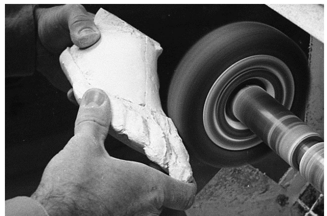
60 Take some off the upper metatarsal to toe joint area. Otherwise, this area will end up too full of extra space inside the footwear.
