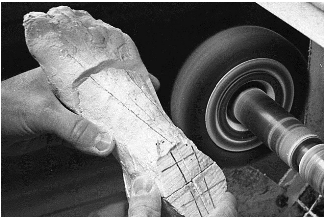
51 This is a coarse wire brush. The objective is to size it all uniformly and make it all smooth. If your skills are not good with the machine, you can probably do a lot better work by hand, it just takes longer.
