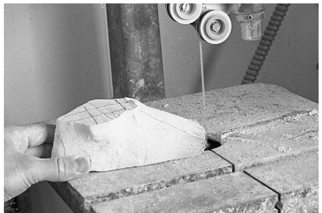
18 Making a center cut on top.
